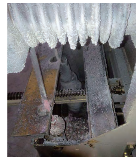
铁磁谐振导致PT粉碎性爆炸
